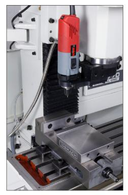
KRESS 800 WATT HIGH SPEED SPINDLE KIT AND 5" CNC VISE FOR WORKHOLDING
