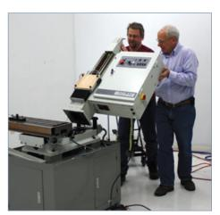
A PATENT-PENDING MOVING KIT MAKES DISASSEMBLY OF THE PCNC 770 SAFER AND EASIER.
